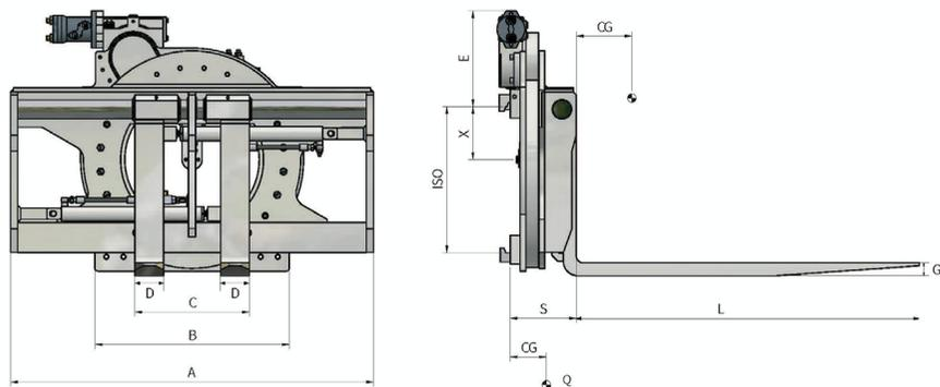
FONCTIONS HYDRAULIQUES: 2 | PRESSION MAX D'UTILISATION: 175 Bar
