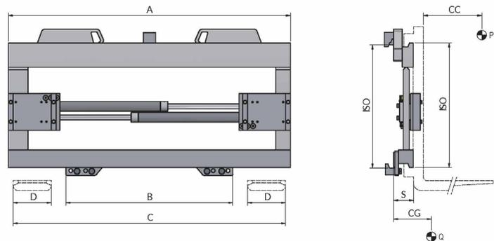
FONCTIONS HYDRAULIQUES: 1 | PRESSION MAX D'UTILISATION: 110 Bar
