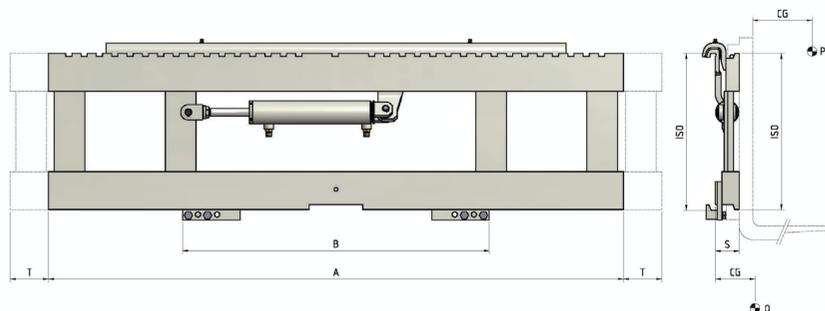
FONCTIONS HYDRAULIQUES: 1 | PRESSION MAX D'UTILISATION: 200 Bar
