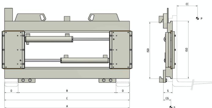
FONCTIONS HYDRAULIQUES: 1 | PRESSION MAX D'UTILISATION: 80 Bar
