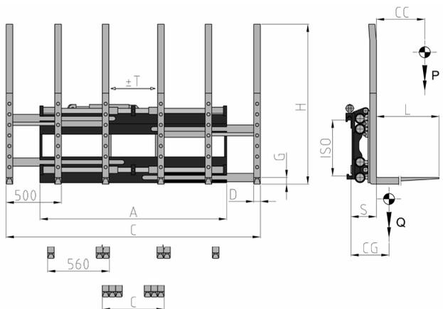
FONCTIONS HYDRAULIQUES: 2 | PRESSION MAX D'UTILISATION: 200 Bar
