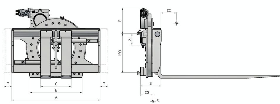
FONCTIONS HYDRAULIQUES: 3 | PRESSION MAX D'UTILISATION: 175 Bar
