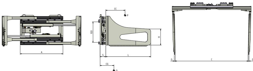
**FONCTIONS HYDRAULIQUES: 1 | PRESSION MAX D'UTILISATION: 175 Bar**
