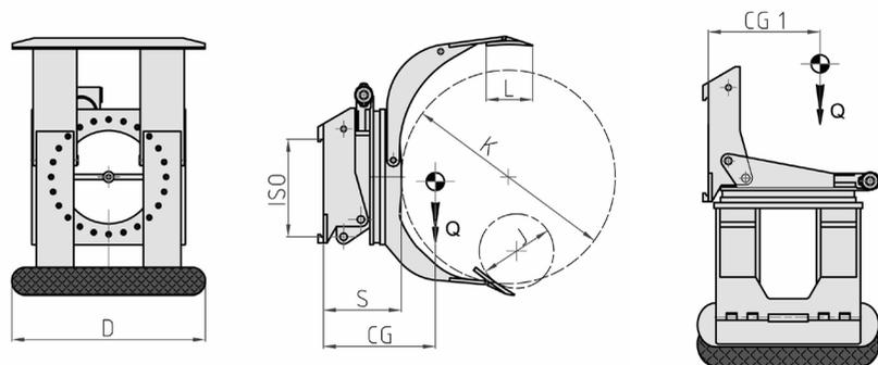
FONCTIONS HYDRAULIQUES: 3 | PRESSION MAX D'UTILISATION: 175 Bar
