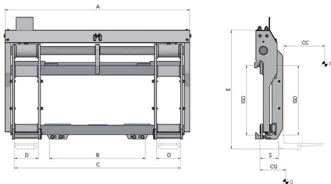
FONCTIONS HYDRAULIQUES: 1 | PRESSION MAX D'UTILISATION: 110 Bar
