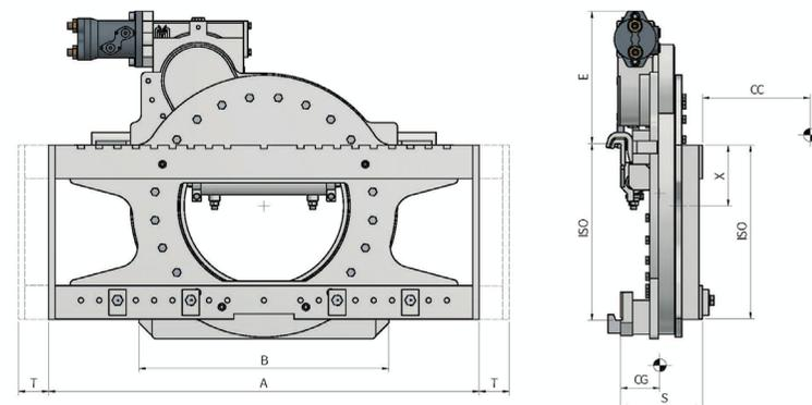
FONCTIONS HYDRAULIQUES: 2 | PRESSION MAX D'UTILISATION: 175 Bar
