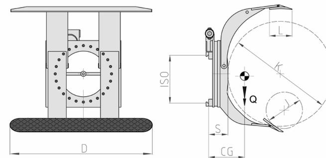
FONCTIONS HYDRAULIQUES: 2 | PRESSION MAX D'UTILISATION: 175 Bar
