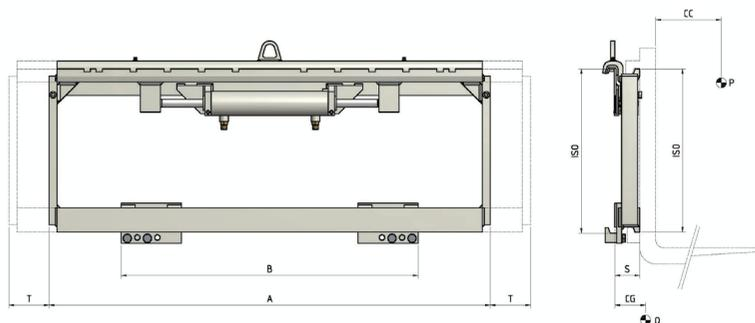
FONCTIONS HYDRAULIQUES: 1 | PRESSION MAX D'UTILISATION: 200 Bar
