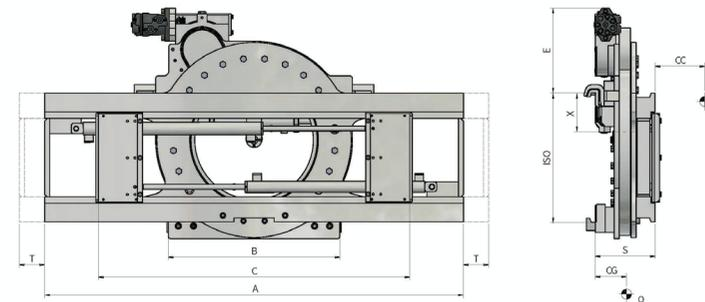
FONCTIONS HYDRAULIQUES: 3 | PRESSION MAX D'UTILISATION: 175 Bar
