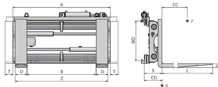
FONCTIONS HYDRAULIQUES: 2 | PRESSION MAX D'UTILISATION: 80 Bar
