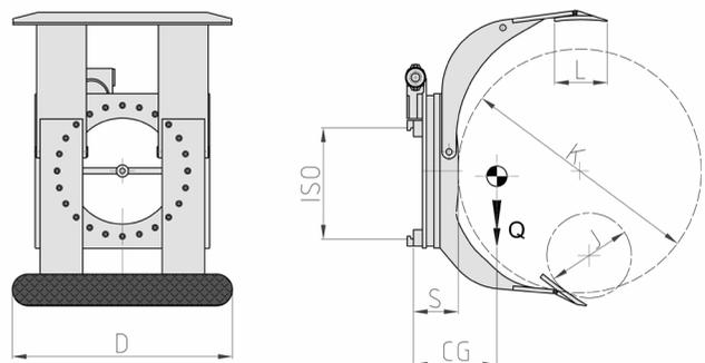
FONCTIONS HYDRAULIQUES: 2 | PRESSION MAX D'UTILISATION: 175 Bar
