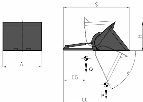
FONCTIONS HYDRAULIQUES: 1 | PRESSION MAX D'UTILISATION: 175 Bar
