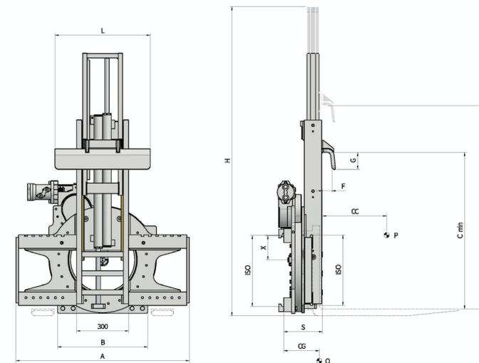
FONCTIONS HYDRAULIQUES: 2 | PRESSION MAX D'UTILISATION: 175 Bar
