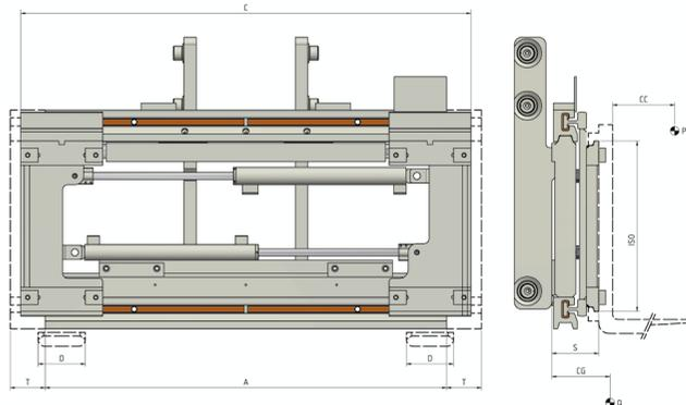
FONCTIONS HYDRAULIQUES: 2 | PRESSION MAX D'UTILISATION: 80 Bar
