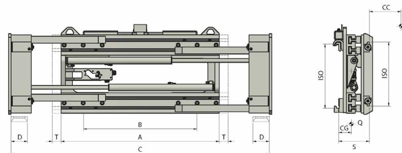
**FONCTIONS HYDRAULIQUES: 2 | PRESSION MAX D'UTILISATION: 80 Bar**
