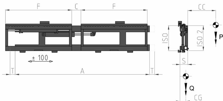
FONCTIONS HYDRAULIQUES: 2 | PRESSION MAX D'UTILISATION: 200 Bar
