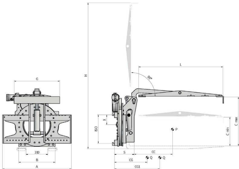
FONCTIONS HYDRAULIQUES: 2 | PRESSION MAX D'UTILISATION: 175 Bar
