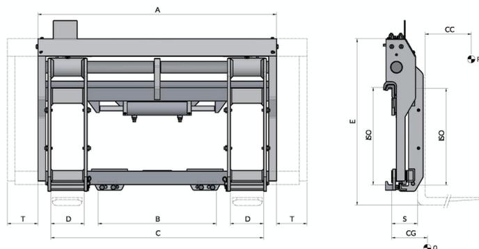
FONCTIONS HYDRAULIQUES: 2 | PRESSION MAX D'UTILISATION: 110 Bar
