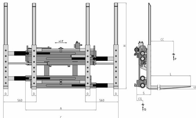
FONCTIONS HYDRAULIQUES: 2 | PRESSION MAX D'UTILISATION: 200 Bar
