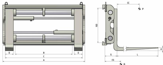
**HYDRAULIC FUNCTIONS: 1 | MAX WORKING PRESSURE: 80 Bar**
