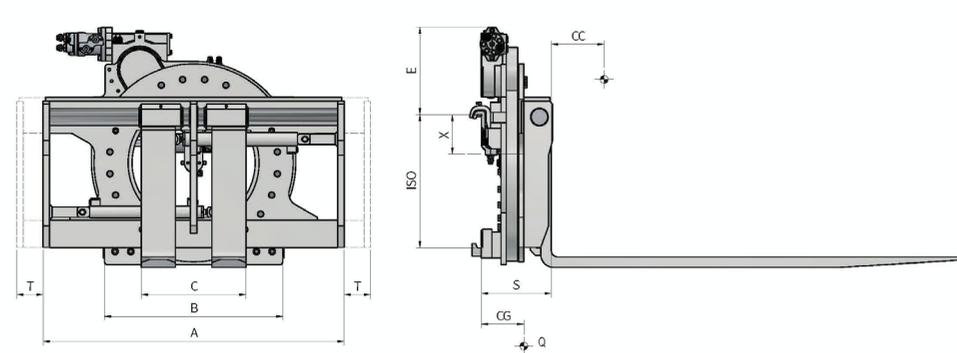
HYDRAULIC FUNCTIONS: 3 | MAX WORKING PRESSURE: 175 Bar
