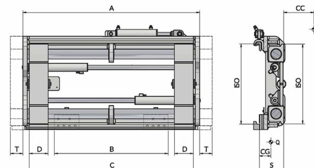
HYDRAULIC FUNCTIONS: 2 | MAX WORKING PRESSURE: 80 Bar
