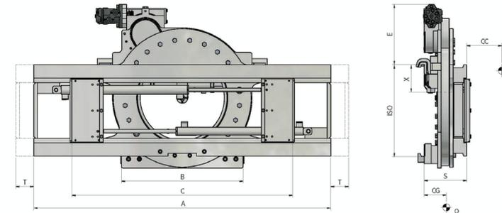
HYDRAULIC FUNCTIONS: 3 | MAX WORKING PRESSURE: 175 Bar
