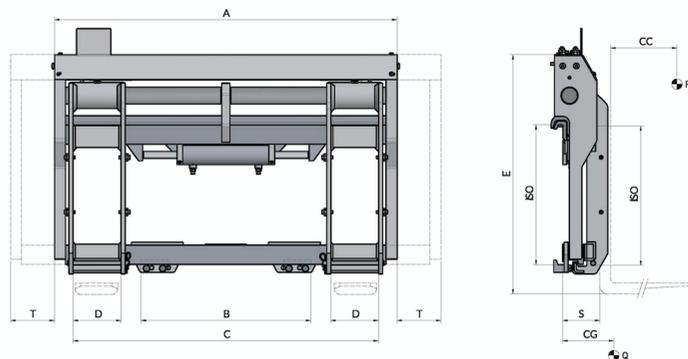
HYDRAULIC FUNCTIONS: 2 | MAX WORKING PRESSURE: 110 Bar
