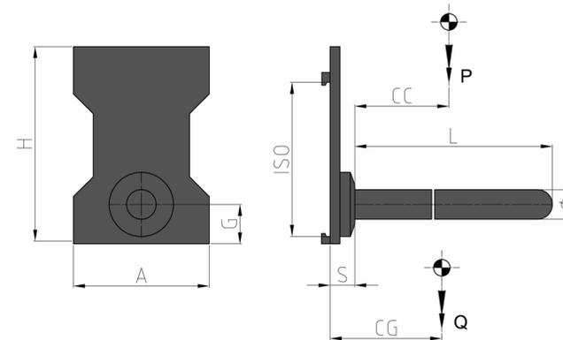
Features: • Grip of tubular loads lying longitudinally to the forklift (paper rolls, carpets, moquette, pipes of plastic, concrete or iron, wire rod rolls). • It can be easily installed on the original Fork Carriage of the Forklift.
