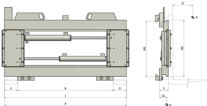
HYDRAULIC FUNCTIONS: 1 | MAX WORKING PRESSURE: 80 Bar
