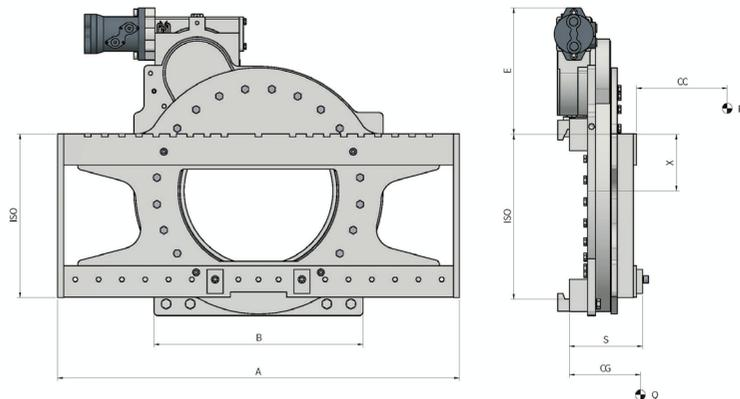
HYDRAULIC FUNCTIONS: 1 | MAX WORKING PRESSURE: 175 Bar
