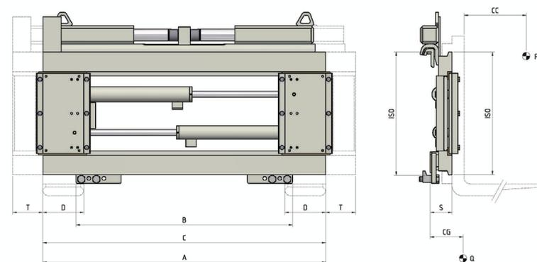
HYDRAULIC FUNCTIONS: 2 | MAX WORKING PRESSURE: 80 Bar
