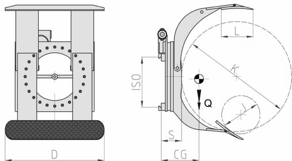
HYDRAULIC FUNCTIONS: 2 | MAX WORKING PRESSURE: 175 Bar
