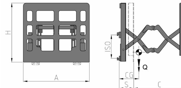
HYDRAULIC FUNCTIONS: 1 | MAX WORKING PRESSURE: 175 Bar
