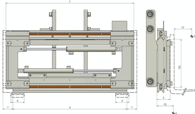
**HYDRAULIC FUNCTIONS: 2 | MAX WORKING PRESSURE: 80 Bar**
