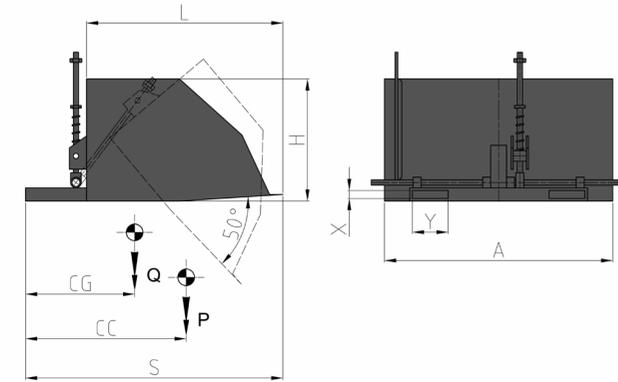
**Features:** • Fork mounted attachment. • Materials loading/unloading operations for Building Industry (sand, gravel, concrete, terrain). • Can also be used in Agriculture. • Suitable for occasional/seasonal work.
