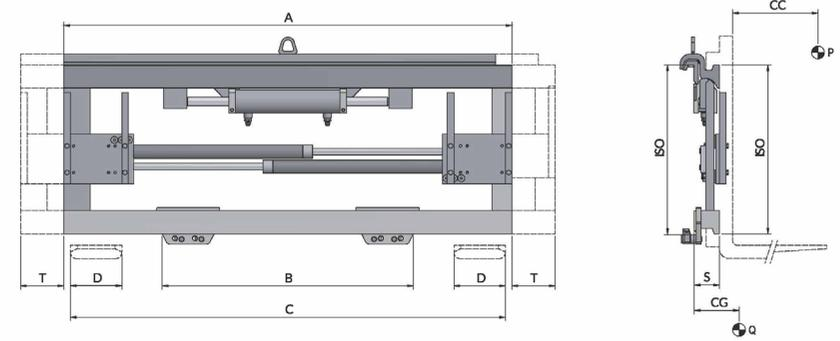
HYDRAULIC FUNCTIONS: 2 | MAX WORKING PRESSURE: 110 Bar
