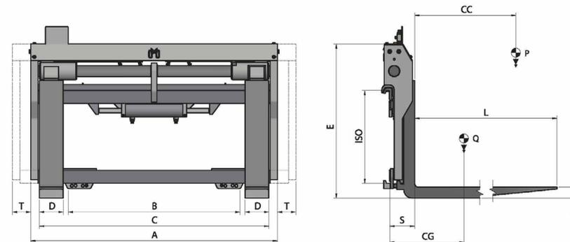
HYDRAULIC FUNCTIONS: 2 | MAX WORKING PRESSURE: 110 Bar
