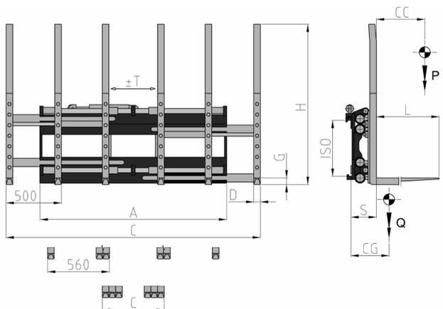
HYDRAULIC FUNCTIONS: 2 | MAX WORKING PRESSURE: 200 Bar
