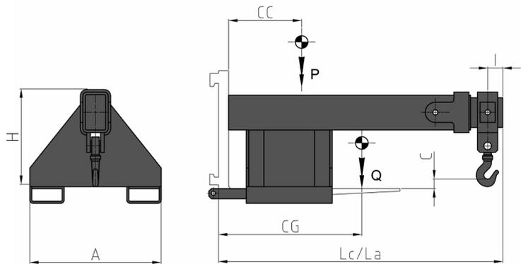
Features: • Fork mounted attachment. • Handling suspended loads. • Use of Belts or Chains.
