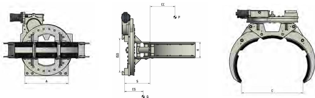
HYDRAULIC FUNCTIONS: 2 | MAX WORKING PRESSURE: 175 Bar
