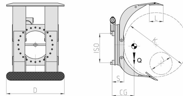
HYDRAULIC FUNCTIONS: 2 | MAX WORKING PRESSURE: 175 Bar
