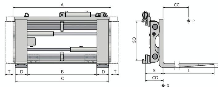
**HYDRAULIC FUNCTIONS: 2 | MAX WORKING PRESSURE: 80 Bar**
