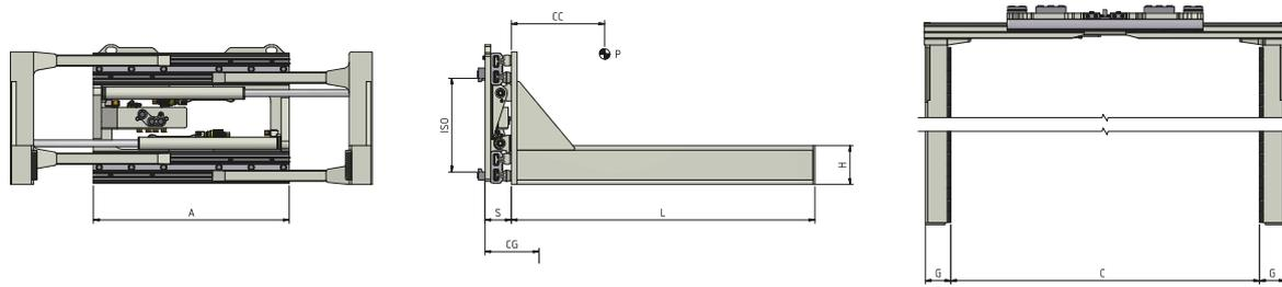
FONCTIONS HYDRAULIQUES: 1 | PRESSION MAXI D'UTILISATION: 175 Bar
