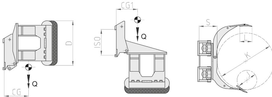
FONCTIONS HYDRAULIQUES: 2 | PRESSION MAXI D'UTILISATION: 175 Bar
