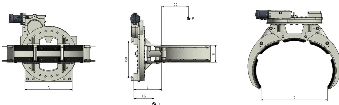
FONCTIONS HYDRAULIQUES: 2 | PRESSION MAXI D'UTILISATION: 175 Bar
