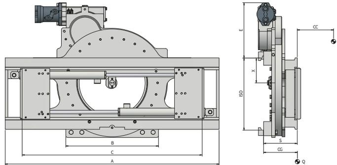
FONCTIONS HYDRAULIQUES: 2 | PRESSION MAXI D'UTILISATION: 175 Bar
